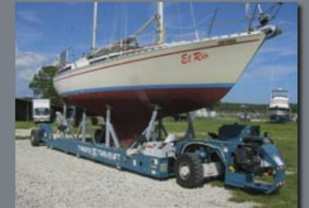
Flexibility for Large or Small Marinas. Our transporters are highly flexible in their lifting options and are perfect for multiple applications. They allow power boats to be lifted by hydraulic lifting supports or sailboats to be lifted on cradles or with out the cradles using the hydraulic lifting supports.
