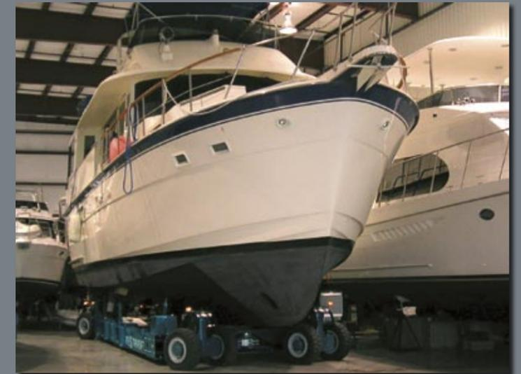
The open-end design permits the lifting of a boat directly from its storage position onto the transporter without a pre-lift. Design innovation like this ensures that our transporters will become a vital tool in the productive operation of your yard.
